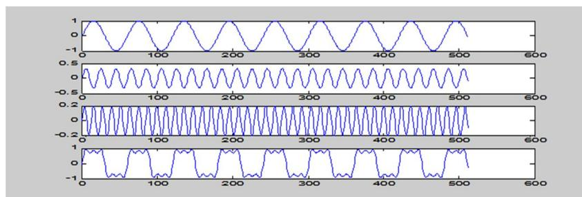
Fig. 7: A 50 Hz signal with harmonics (fourth signal) obtained by superposition of first three signals in MATLAB
