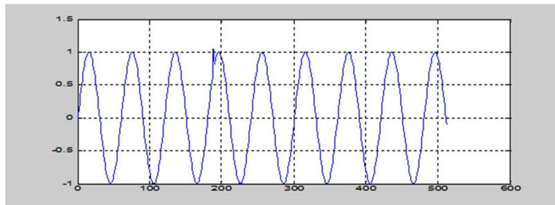
Fig. 9: A 50 Hz signal with oscillatory transient obtained by MATLAB simulation
