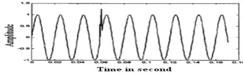
Fig. 2: A 50 Hz fundamental signal with an impulse presented in the literature [3]
