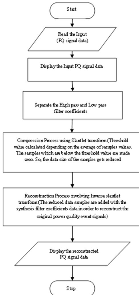
Fig. 4: Flowchart explaining computer procedure adopted for compressing data pertaining to a power quality event using slantlet transform method and subsequent reconstruction of the power quality signal
