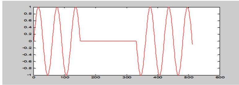
Fig. 8: A 50 Hz signal with momentary interruption obtained upon MATLAB simulation
