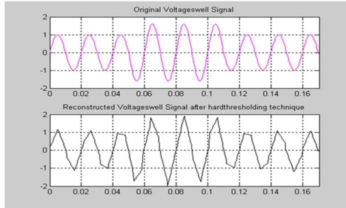
Fig. 11: Original voltage swell signal and reconstructed swell signal with compression ratio equal to 10
