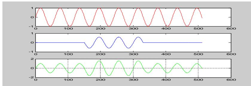
Fig. 6: A 50 Hz signal with voltage swell (third signal) obtained by superposition of the first two signals upon MATLAB simulation
