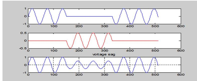
Fig. 5: A voltage sag signal (third signal) obtained by superposition of the first two signals upon MATLAB simulation
