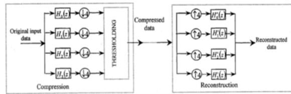
Fig. 1: Two-scale slantlet transform based scheme for data compression and reconstruction adopted in the present work
