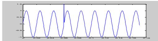
Fig. 3: A 50 Hz fundamental signal with an impulse obtained by MATLAB simulation in the present work
