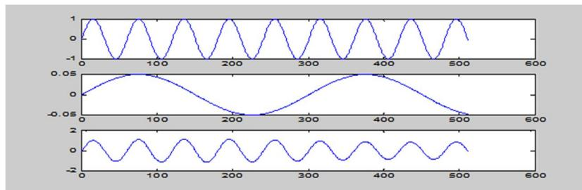
Fig. 10: A 50 Hz signal with voltage flicker (third signal) derived from the first two signals obtained by *MATLAB* simulation
